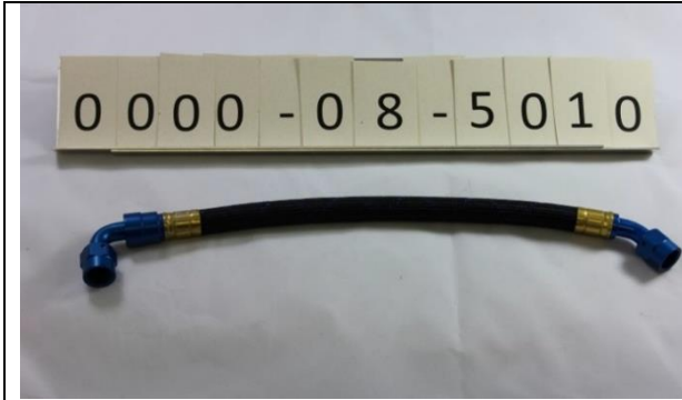
RE-Cooler to Housing Line 0000-08-5010
