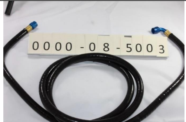
Trans - Cooler to Housing Line 0000-08-5003
