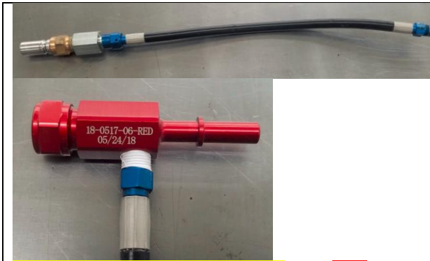
Fuel Pump Out Kit 0000-06-5210 Only RED fuel tee is allowed, black tee must NOT be used
