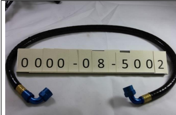
Oil Cooler to Engine Line 0000-08-5002
