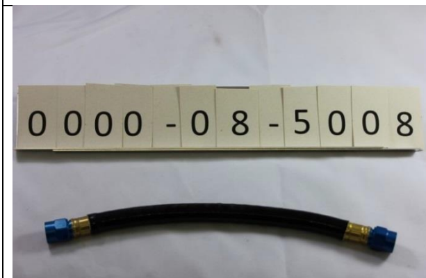
RE-Filter to Pump Line 0000-08-5008
