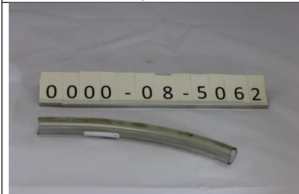
Fuel Tube, 1" Tygon Tubing 0000-08-5062
