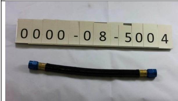
Trans-Housing to Filter Line 0000-08-5004
