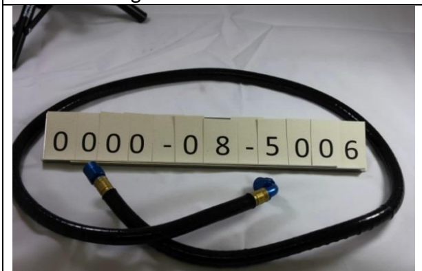
Trans-Pump to Cooler Line 0000-08-5006
