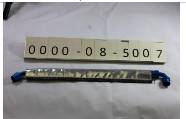
RE-Housing to Filter Line 0000-08-5007
