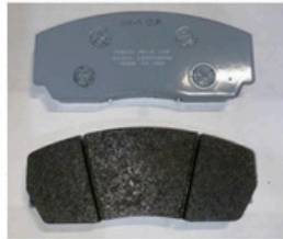
PAGID Front Brake Pads (MX-5C Required) 0000-03-5106-61
