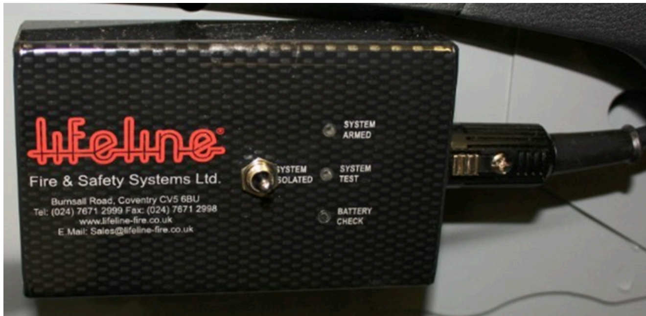
Figure 4: Fire System Control Unit, Right Side of Center Console.
