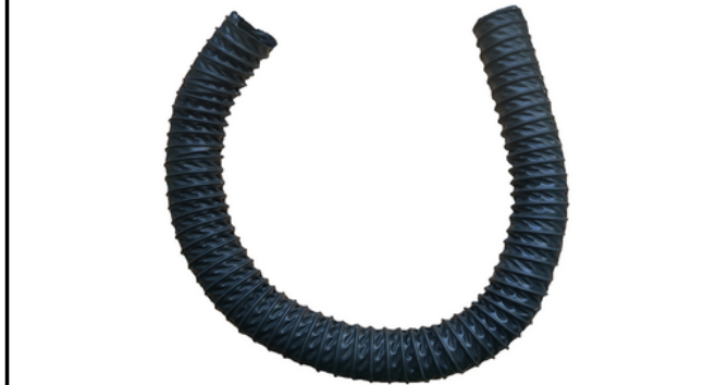
(Dual) 2" Brake Duct Hose 0000-03-5601-HS-A (Dual 39") (Alternative - Optional)
