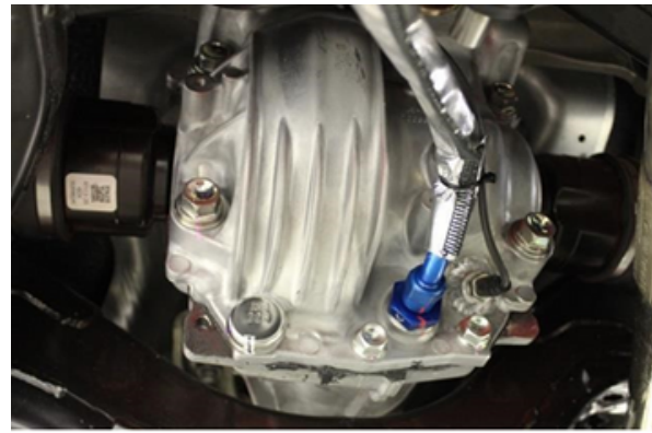
Diff Cover, Bottom with Temperature Sensor 0000-08-5033
