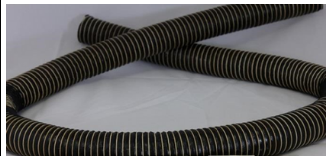
(Dual) 2" Brake Duct Hose 0000-03-5601-HS (Dual 39") (Optional)
