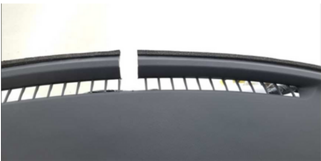
Trim dash to allow clearance for windshield brace and bracket.
