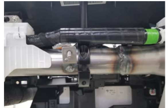
Attach brace support bracket to dash bar
