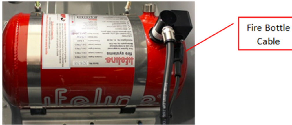
Figure 3. Fire Bottle Cable, Trunk.
