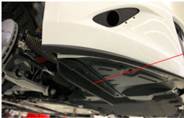
Figure 9: Plastic Angles Excluded from Ride Height Measurement
