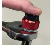
The knobs will come loose, but the hex shaped adjusters should stay with the shaft. As seen below, the two hex shapes may need to be aligned to remove the knobs completely.
