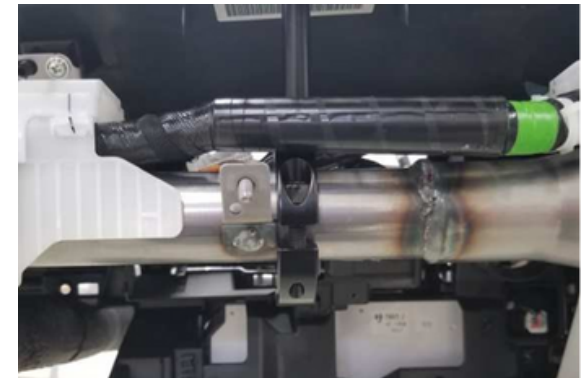
Attach brace support bracket to dash bar
