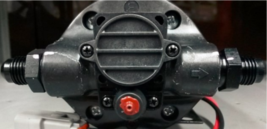
Figure 15: Transmission and Differential Cooling Pump
