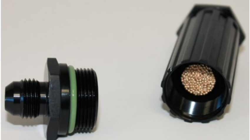
Figure 16: Transmission and Differential Cooler Line Filter, Disassembled
