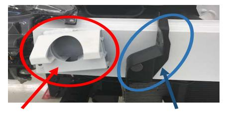
Right & Left protrusions that must be removed
