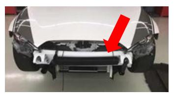
Remove the Right and Left Protrusion and the Air Guide.
