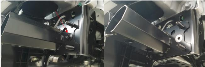
2.4 Install Fascia Support Bracket over studs on frame horn, line studs up with the bottom of the slots in the Fascia Support and install two M8x1.25 Flange Nuts (14ft-lbs).
