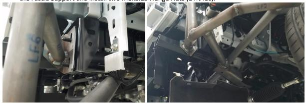
2.5 Install two M6x1x16 Flange Bolts (7ft-lbs) securing the under-tray and Fascia Support together to the subframe.
