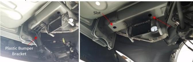
2.4 Remove tape covering factory holes on the outer side of the Rear Frame Rail, and prepare the two holes shown for weld.
