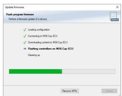
8. When firmware update is complete, click ok, then turn Vehicle power off, then back on to power cycle the ECU.
