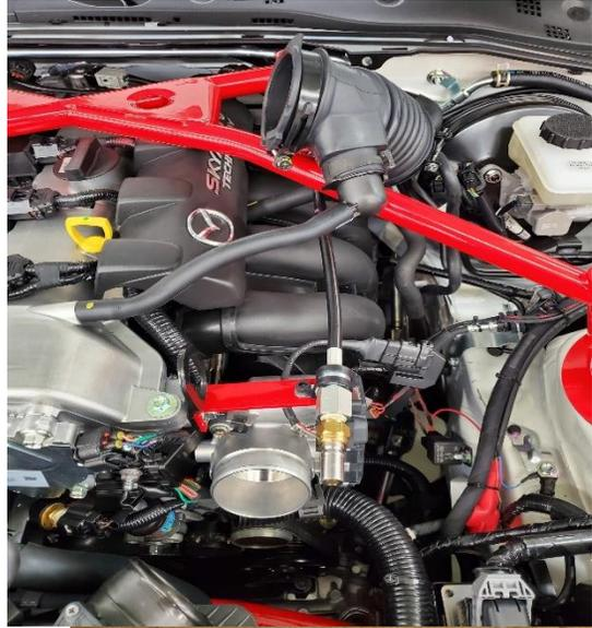
2.3 Using an 8mm socket, remove the four bolts on the front side of the throttle body.
