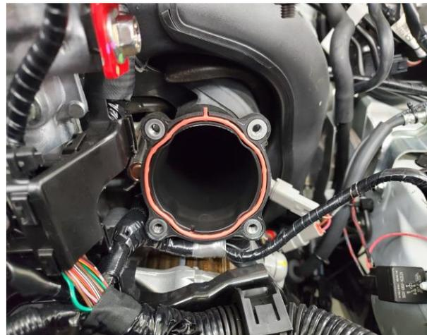
3.5 **Note:** ND2 throttle bodies have 3 short bolts and 1 long bolt. Included in the kit are 3 more long bolts. You will need 4 long bolts to install your Bosch throttle body.
