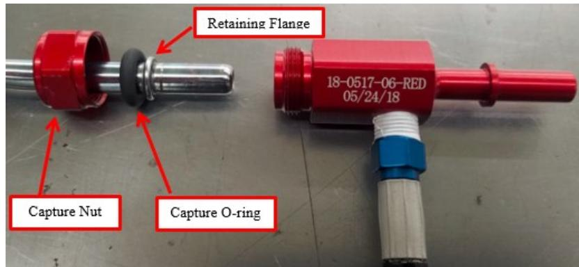
4. Lubricate the outer surface of the fuel line with a silicon O-ring lubricant and then slide the Fuel Line Adaptor over the fuel line. Tighten Capture Nut to body and connect fuel line.
