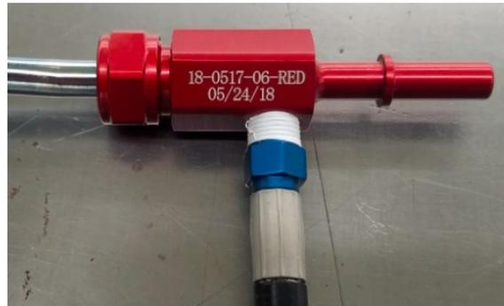
5. Turn power on vehicle and inspect for leaks. If no leaks are present start vehicle and inspect for leaks while running. Do not continue use with any sign of leaks present.
